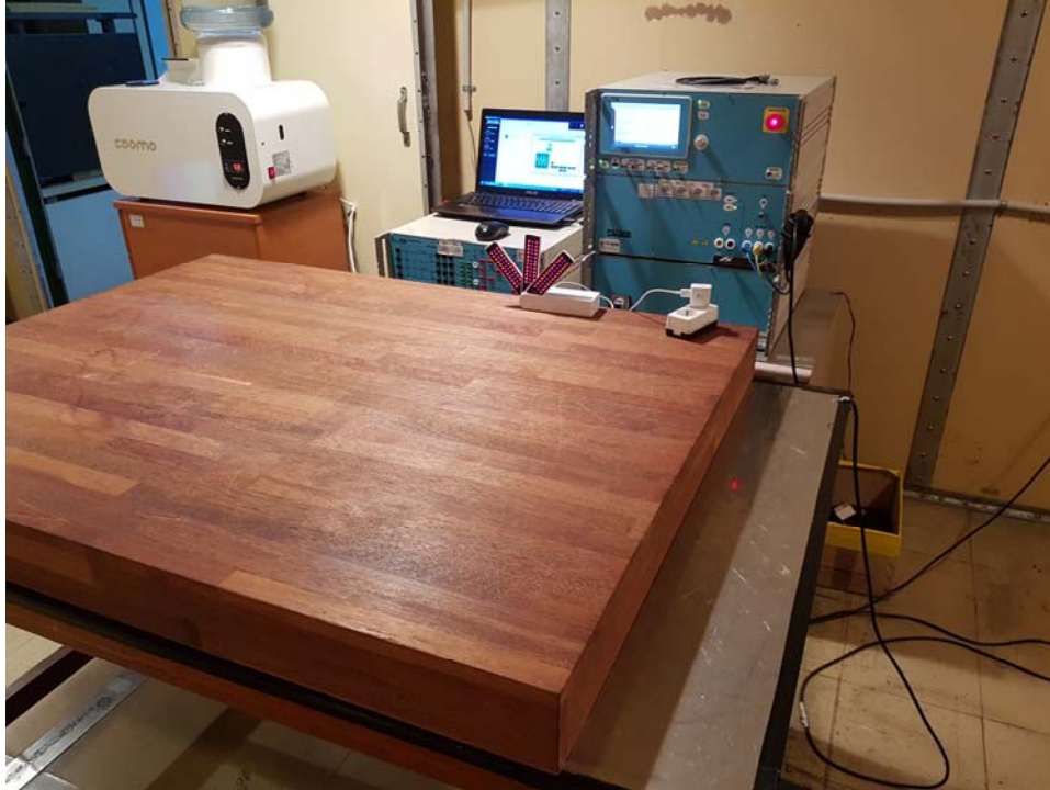
[Voltage Dips and Voltage interruptions immunity Test]
